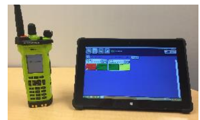
APX-turned-RF Modem Connects to a Tablet PC Running APAA via a Data Interface Cable (left) or via Bluetooth (right)
