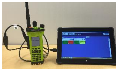
APX-turned-RF Modem Connects to a Tablet PC Running APAA via a Data Interface Cable (left) or via Bluetooth (right)
