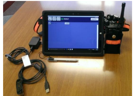
Portable APX Radio Configured As RF Modem Enables Untethered Fireground Accountability Operations
